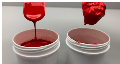
30% ZETASPERSE® 3800 (left) and 30% Competitor (right) in water, calculated on PR 112
