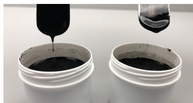
56% ZETASPERSE® 3800 (left) and 56% Competitor (right) in water, calculated on PBk7
