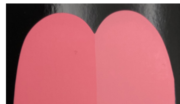
30% ZETASPERSE® 3800 (left) and 30% Competitor (right) in water, calculated on PR 112
